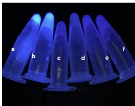
Figure 6: Naked-eye detection for analyzing PBA-OH interaction with dopamine (DA) at varying concentrations in artificial sweat as the following: no addition of DA (a), 5 \times 10^{-3} M mol (b), 1 \times 10^{-2} M (c), 1.5 \times 10^{-2} M (d), 2 \times 10^{-2} M (e), and 2.5 \times 10^{-2} M (f). Under 365 nm black light.
